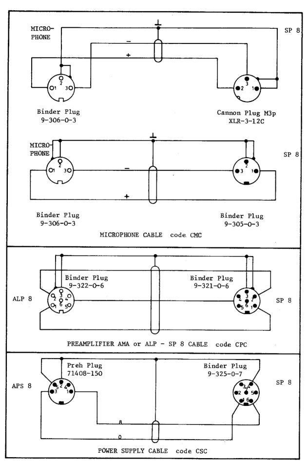
Note: All lengths (unless indicated) must be ordered as additional figure to the code number. Standard cable lengths: 1,5/3/5 and 10 meters.
